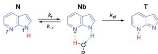
Scheme 1. The widely discussed ESDPT mechanism of 7AI in alcohols (ROH) and water. In this study Nb is directly photo-generated from the ground state.
